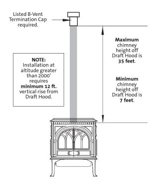
Listed B-Vent Termination NOTE: Cap required. Installation at altitude greater than 2000' Maximum total requires horizontal minimum 12 ft. anywhere in vertical rise from venting configuration Draft Hood. is **4 feet.** Minimum chimney height from Draft Hood is 7 feet. Max. Four, 45° or Three, 90° Elbows
